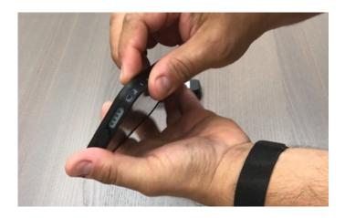
Carefully check that the seal is complete the whole way round the join
