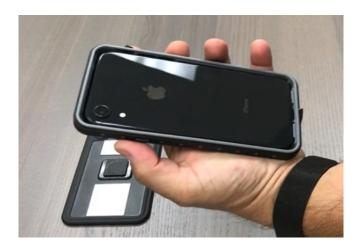
Place the iPhone into the top case with the screen facing down and ensure it is fully inserted.
