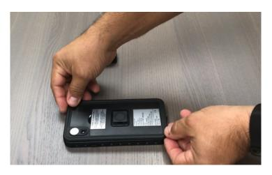
Place bottom case onto top case and ensure aligned correctly
