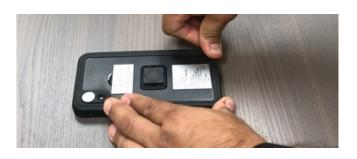
Push down hard to seal the two case halves. Start in on corner and work round the case until fully sealed
