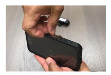
Finally attach the Warranty void labels over the seam between top and bottom
