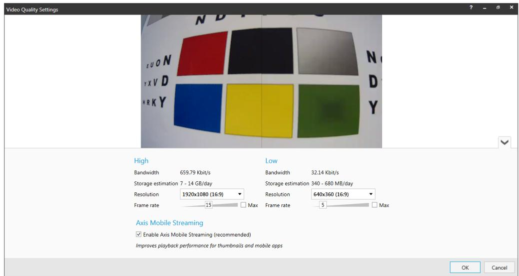
Figure 3: Profile configuration for Axis Mobile Streaming.
