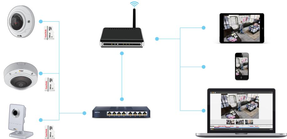
Figure 2: A typical AXIS Camera Companion system setup.
