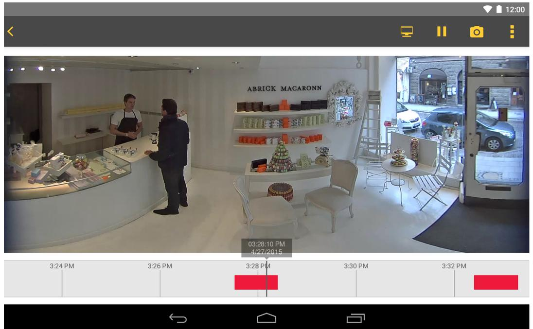
Figure 4: Example of a surveillance situation viewed in high quality. The red color indicates a recording that is triggered by video motion detection.
