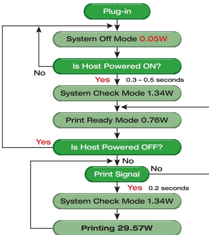
Those clever engineers at Star have designed this printer to correspond directly to the PC it has been attached to. Users will first of all notice that there is no power switch and that the printer can only be turned on by actually attaching the included USB cable to the printer and PC / terminal. The printer will only activate when the PC / terminal is powered up otherwise it can remain in standby mode, thus saving power.
