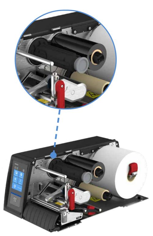
Ribbon Rewind - Small Collapsible Core
