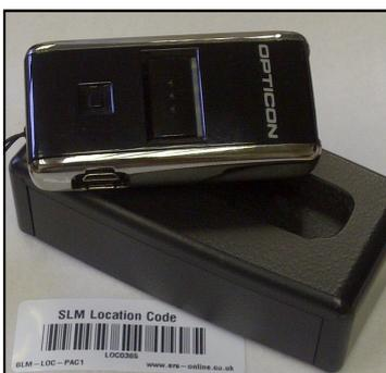
Patrols or attendance are monitored by scanning barcode location labels and incident or observation codes with the keyfob data collector. The date/time tagged transactions will be stored in the data collector and may be downloaded to the system database via USB for subsequent reporting and analysis.
