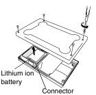
**3** Disconnect the connector, and then remove the lithium ion battery.
