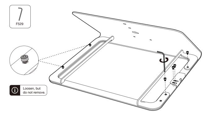
3 Remove right-hand tablet bracket and cord securer
