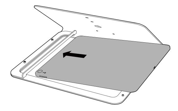
5 Route your USB-C cable and reinstall right-hand tablet bracket
