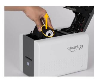
Figure 10 Take out the ribbon cartridge
