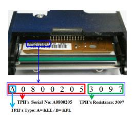
Figure 67 Thermal Print Head
