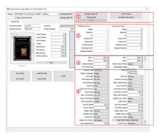
Figure 53 CardPrinterConfig - Card Printer Advanced Setup
