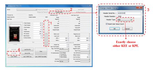
Figure 68 Print head setup
