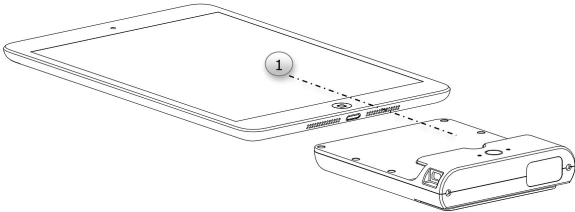
2. Gently slide the Infinea TAB M into position as shown below.
