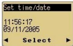
Change the time and date. The changed time and date is stored when the CLR key is pressed. This options only works on the OPL9728 and not on the PC.
