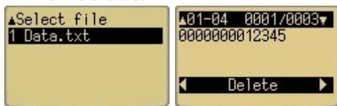
With browse data option it is possible to look through the records and fields of the data file. First the data file to browse needs to be selected. Only one of the data fields is shown on the display at the time. The two number on the top left of the display show the amount of fields that are in the data file. The two number on the top right show the amount of records in the data file. By pressing the CLR key the user return to the Utilities menu.
