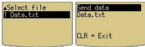
Send data starts the file selection to transfer one or more data files. The protocol for transmitting the data file to the PC is the standard Opticon NetO protocol. To receive the file on the PC an application is needed. The NetO protocol application can be downloaded from the [www.opticon.com](http://www.opticon.com) web site.
