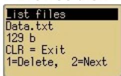
Browses the contents of the RAM disk. With the CLR key the interpreter returns to the Utilities menu. with the 1 key the file can be deleted. With the 2 key the OPL9728 continues to the next file, after the last file the OPL9728 returns to the Utilities menu.
