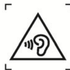
Figure 1 – Warning label (IEC 60417-6044)
