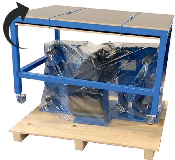
3. Cut the tape and let the lower table top slide down carefully.
