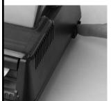
1 Press the Power Switch to the ON position.
