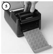
**NOTE:** the ribbon text on the leader should be face down in front of the printer as shown.
