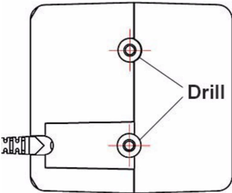
**Figure 2: Mounting Plate Boring Template- Bottom View**
