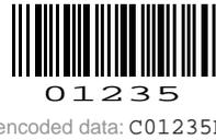
Fig. C.21. Example for Codabar ABC
