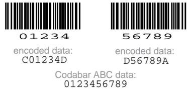
Fig. C.22. Example for Codabar CX
