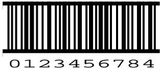
Fig. C.30. Example for MSI/Plessey with MOD 10 Checksum
