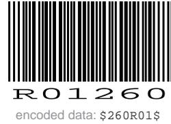
Fig. C.20. Example for Codabar
