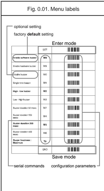
Besides options, some chapters have commands. The commands need to be scanned directly, without reading the "SET" and "END" labels. The commands are executed directly and, unlike options, are not stored in non volatile memory.
